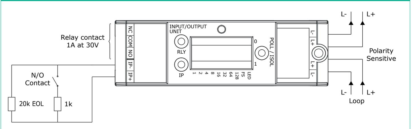
Figure 3 Intelligent Twin Input/Output Unit normally open monitoring mode connectivity diagram (compatible with CoreProtocol only)
