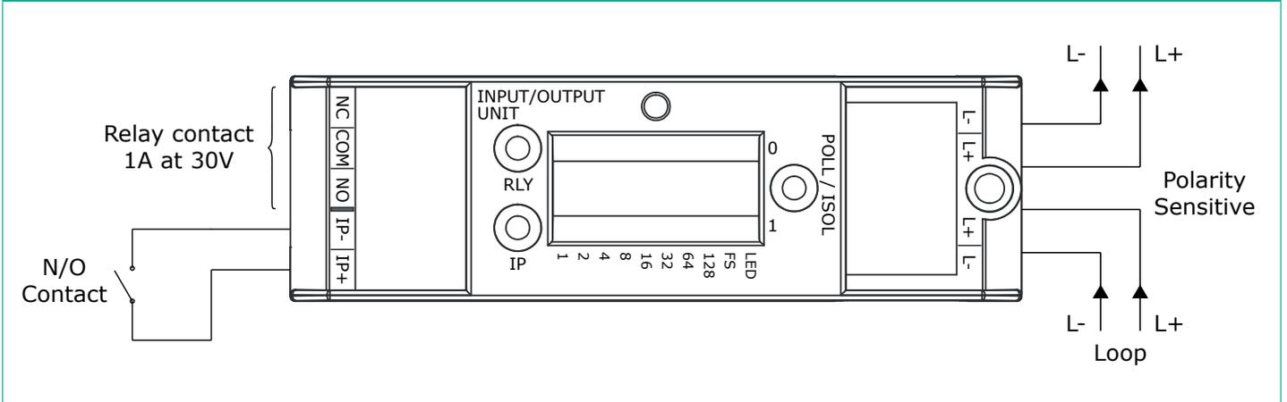
Figure 4 Intelligent Twin Input/Output Unit normally closed monitoring mode connectivity diagram (compatible with CoreProtocol only)
